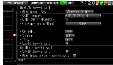
<Access point settings>
