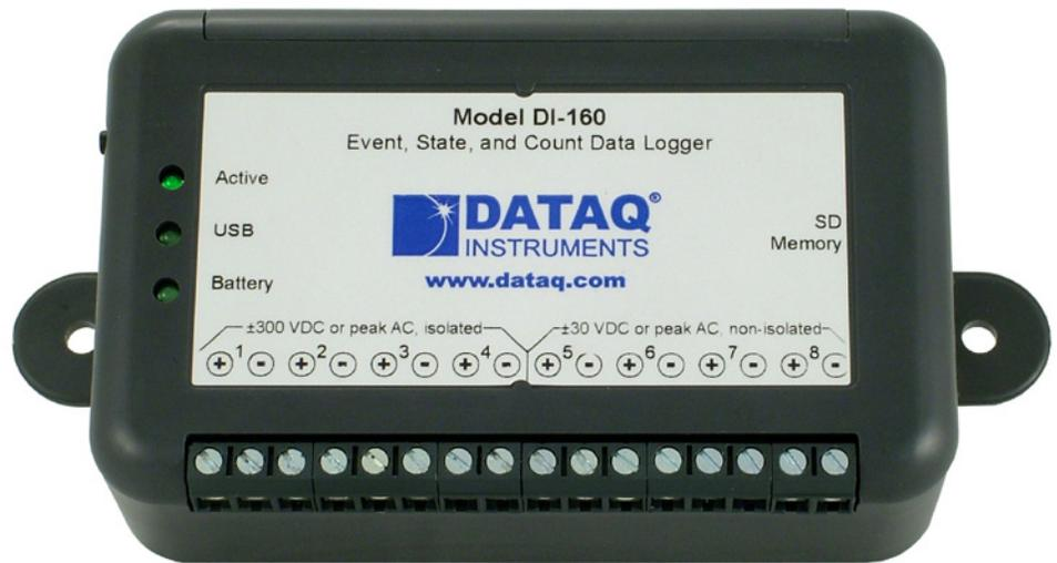
The DI-160 features programmable capture modes to detect events (when the events happen), states (how long between events) and counts (how many events). An internal real time clock provides time and date stamping for each captured quantity, and storage is accomplished to a removable SD-style memory card.
