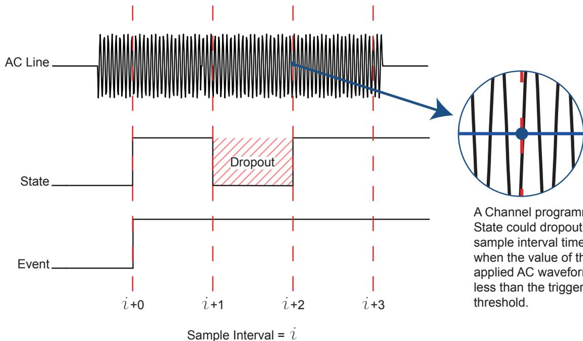
A Channel programmed for State could dropout if the sample interval times out when the value of the applied AC waveform is less than the trigger threshold.
