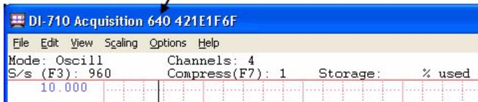
The **Device ID** is the IP address of the instrument. If you are accessing the device over the internet you will also need to enter the Port number designation.
