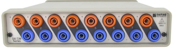
Each of eight fully differential and isolated channels support  $\pm 10 \text{mV}$  to  $\pm 1000 \text{V}$  measurements across six programmable ranges. Access is via recessed banana sockets.
