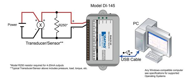
Typical Transducer/Sensors above include pressure, load, torque, Etc.
