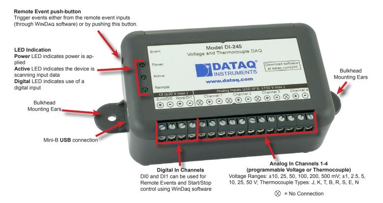
Screw terminals for signal inputs
