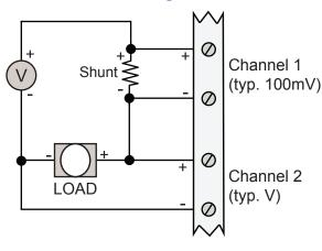
\*Model R250, 250 shunt resistor, see Ordering Guide
