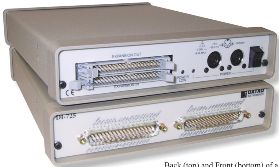
Back (top) and Front (bottom) of a DI-725 analog channel expander.
