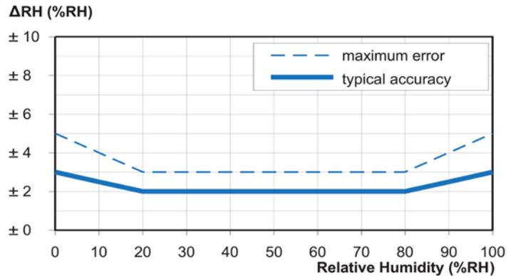
Relative humidity sensor typical accuracy in %RH (0 to 80°C)
