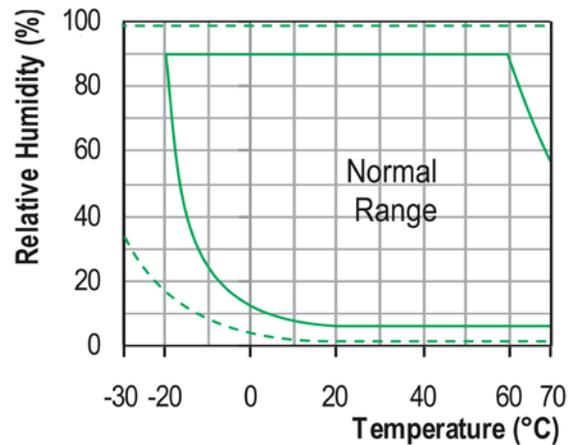
Long term exposure to humidity levels outside of the 'normal' range may temporarily offset RH measurements ( $\pm 3\%$  RH after 60 hours). Once returned to less extreme conditions the device will slowly return to a calibrated state.
