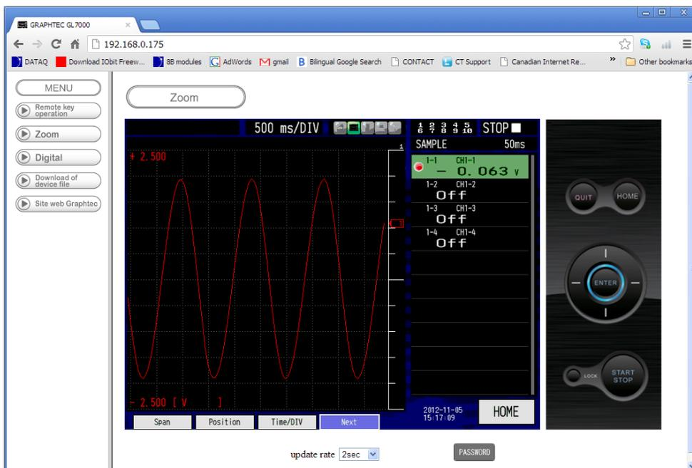
A typical virtual instrument display of the GL7000 using the Chrome browser
