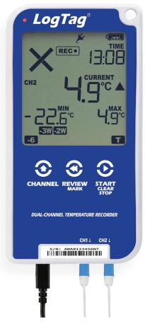
The LogTag® UTRED30-16 Temperature Recorder measures and stores up to a total 32,000 temperature readings. 16,000 readings per channel. The logger supports the ST100 probe and can be used on one or both channels if required.
