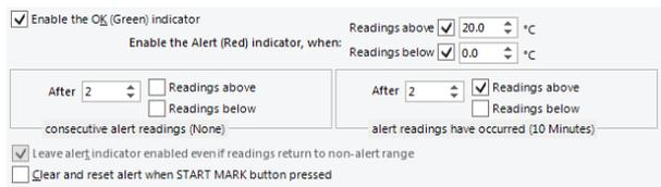
Figure 31: Advanced Alert Settings – Sample settings
