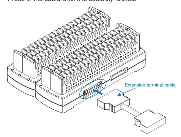
(4) Connect the other end of the extension terminal cable to GL820. \* Press in the cable until it is securely locked.
