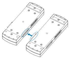
(2) Screw on the connection plate using attached screws. \* Recommended screw torque: 14 kgf/cm
