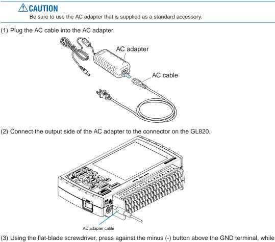
connecting the grounding cable to the GL820. Connect the other end of the cable to ground.
