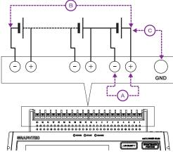
Input Circuit Diagram for Analog Input (Voltage, Thermocouples)
