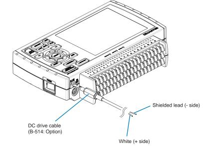
(3) Connect the DC input side to the DC power supply.
