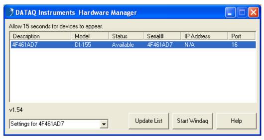
The Hardware Manager allows you to start WINDAQ Acquisition software (select the device and click on the **Start Windaq** button) and must be used when multiple DATAQ Instruments devices are installed. It also provides crucial information about your device needed for custom programming (Serial # and COM Port).
