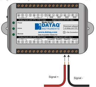
Select Channel 10 in the channel display, then select **Edit** > **Channel Settings** in the menu to specify a full scale range for the Rate channel. Ranges of 5, 10, 20, 50, 100, 200, 500, 1000, 2000, 5000, and 10000 Hz are available. Choose a range that comes closest to your expected full scale rate or frequency. For example, if you need to measure the output of a flow meter that can measure a maximum flow rate of 100 gallons per minute, and the output frequency
