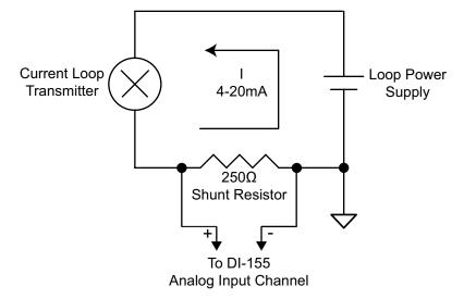
Set the engineering units as desired and define upper/lower levels in WINDAQ as 1V = 4mA for the low value and 5V = 20mA for the high value. For example, when using WINDAQ Acquisition software, in the EU Settings dialog box:
