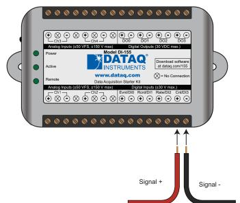
Connect any TTL pulse stream (30 VDC max) to the Cnt/DI3 channel on the DI-155.
