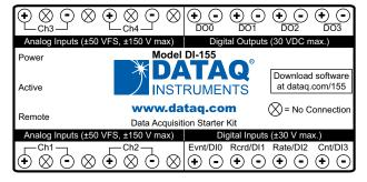
Analog Inputs Ch#: Analog channels 1-4 (±50VFS, ±150V transient max.)
