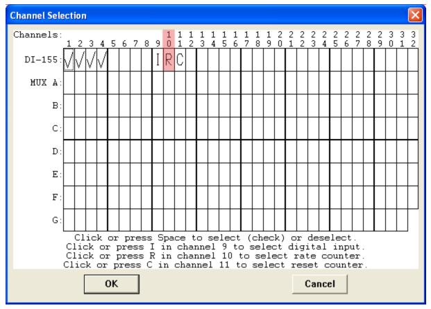
Connect any TTL pulse stream (30 VDC max) to the Rate/DI2 channel on the DI-155.
