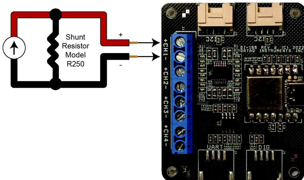
The shunt resistor should be placed on the low side of the circuit as shown below:
