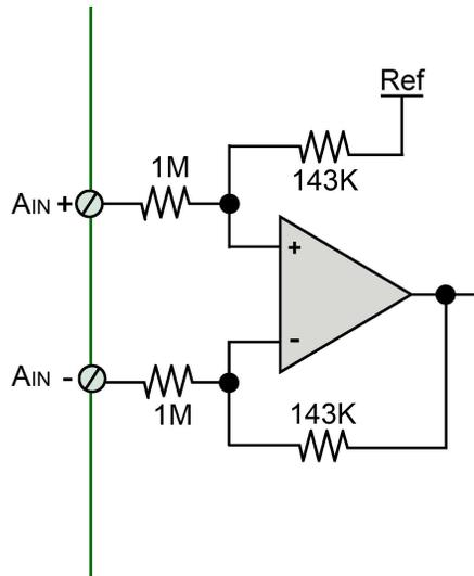
Use the following diagram to connect Analog Input Channel 1.
