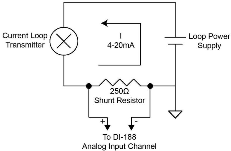
Set the engineering units as desired and define upper/lower levels in WINDAQ as 1V = 4mA for the low value and 5V = 20mA for the high value. For example, when using WINDAQ Acquisition software, in the EU Settings dialog box:
