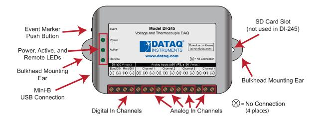
Please note: The SD card slot is not used in the DI-245. Allowing foreign materials to enter the device through the SD card slot may result in damage to the instrument.
