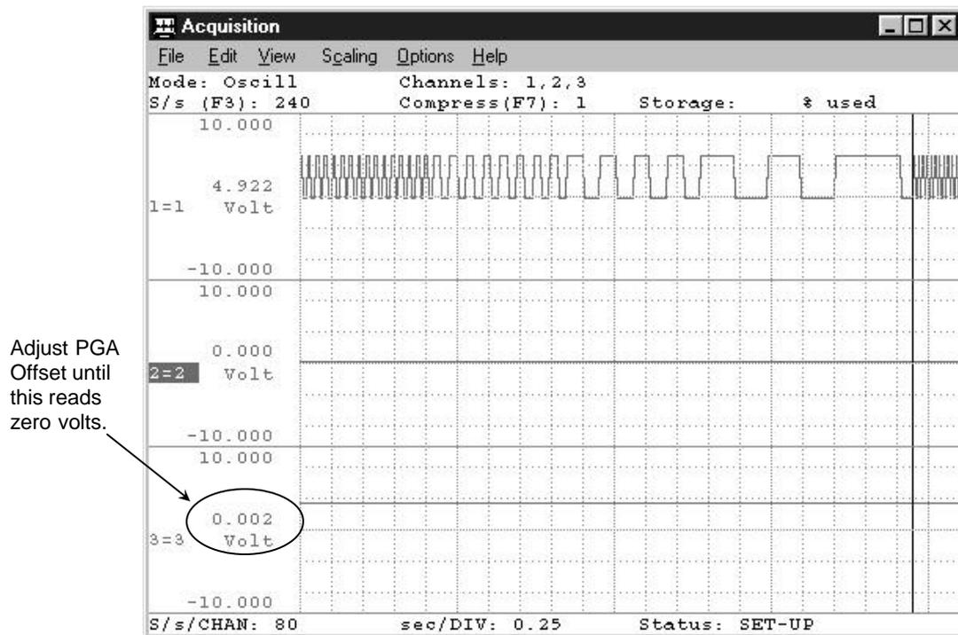
11. Repeat steps 9 and 10 until both channel's numerical display reads zero volts (or as close as possible).
