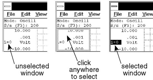
When selected, a box surrounds the variable waveform assignment indicator, indicating that the channel is selected for adjustment.
