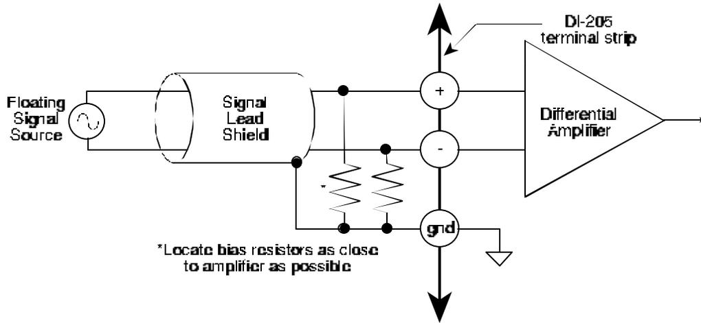
**Signal Cable and the Differential Amplifier**
