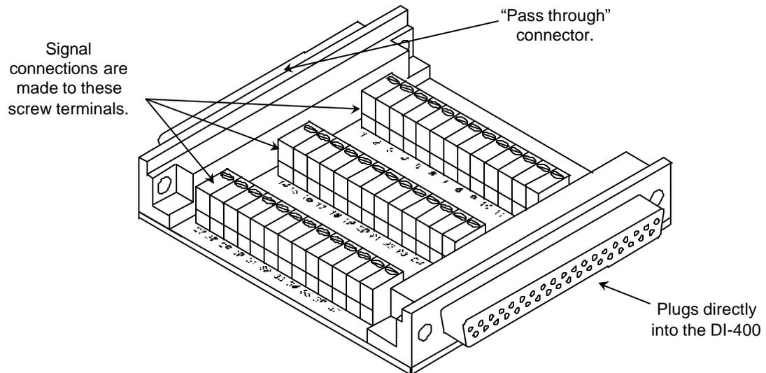
Any combination of single-ended or differential channels may be connected to the DI-705, but keep in mind a differential channel uses two analog inputs. Configure single-ended and differential channels on the DI-705 the same way as on the DI-400. Refer to the paragraph titled “I/O Connector and Signal Connections” in the Specifications section of this manual for single-ended/differential configuration details.
