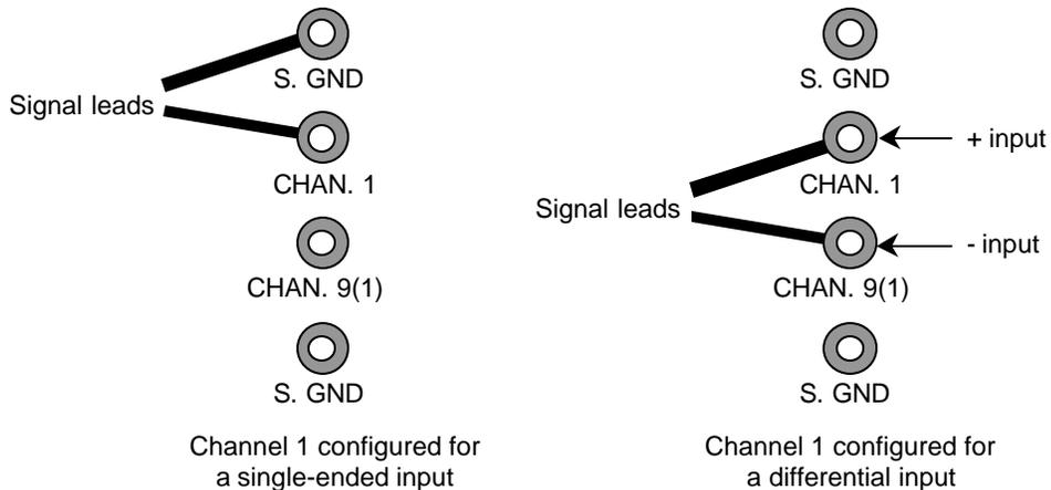
Note that when an input channel is configured for differential operation, the binding post associated with that channel's high (+) input assumes the channel number.
