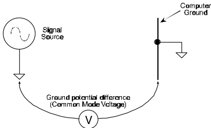
The most common of these is different physical locations of the computer and signal ground points. Since wire is not a perfect conductor (i.e. exhibiting zero resistance regardless of length) a voltage drop, however small, will always be present. The differential amplifier is unique in its ability to measure signals originating from sources with different ground potentials relative to the computer *providing it is connected properly*.
