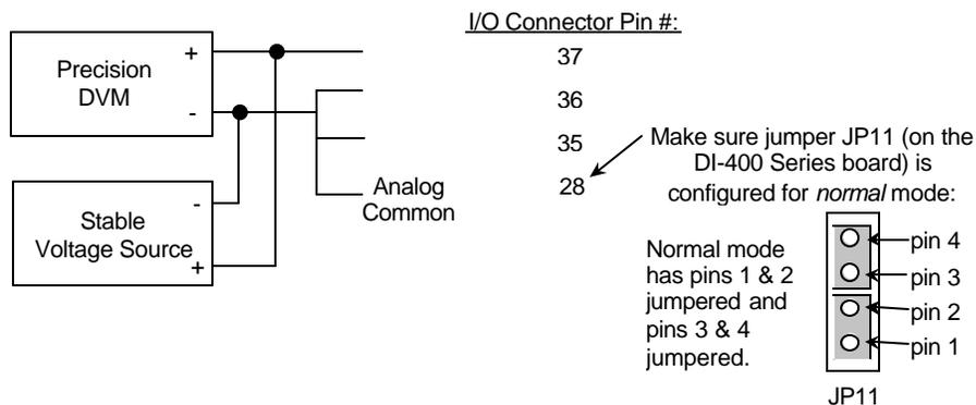
Or if you are using the alternative voltage calibrator, the following figure illustrates the necessary connections:
