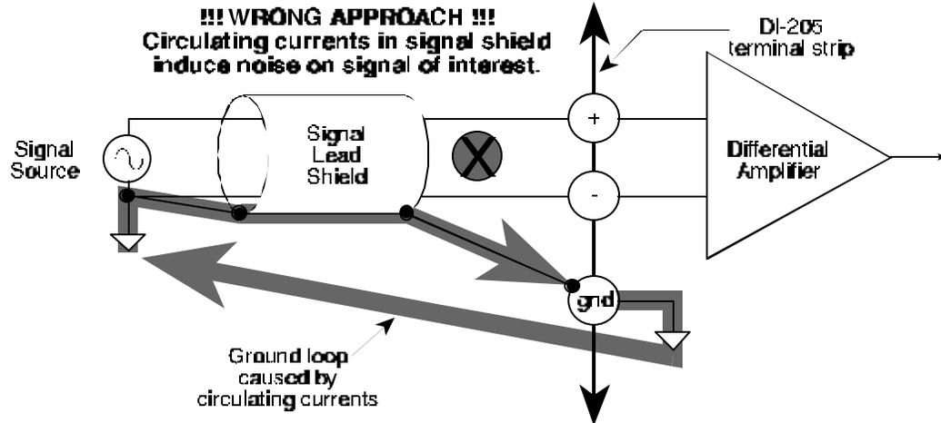
The most common error made in connecting differential amplifiers is the tendency to ground both ends of a signal shield. This causes current to flow through the shield and induces noise on the signal to be measured. This problem is eliminated by ensuring that only one ground exists on the signal circuit.
