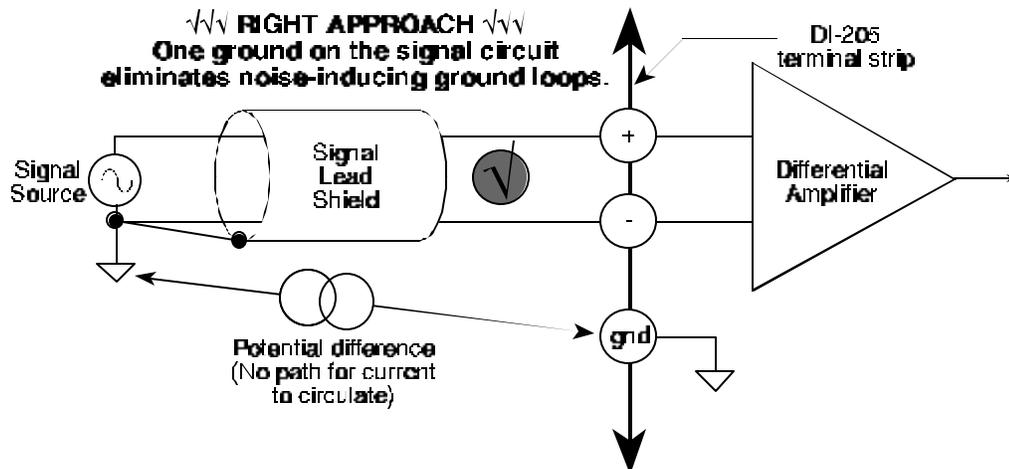
**Isolated Signal Sources** — There are two considerations when connecting a differential amplifier to an isolated signal source: The elimination of ground loops as described above, and the use of bias resistors to provide bias current for the differential amplifier's positive and negative inputs.
