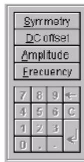
All described functions can also be controlled using the keyboard. When the window is expanded, a small key pad is located which enables entering all settings.
