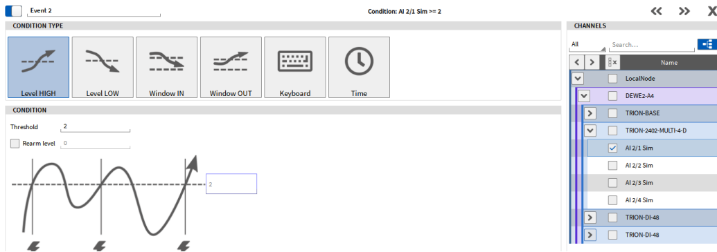
Figure 7-23: Level High Condition Type; Threshold: 2
