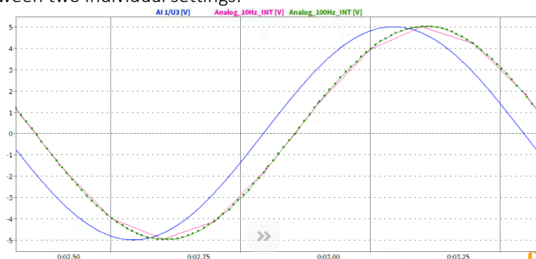
Figure 5-98: Blue: Analog Input; Green: CAN-Output with a delay of 70ms (default value)
