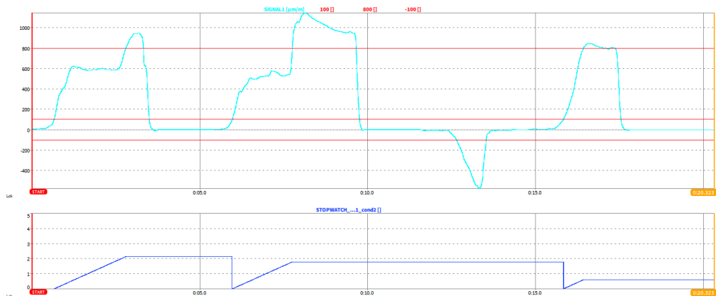
Figure 5-29: Stopwatch with start and stop condition
