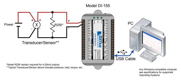
Typical Transducer/Sensors above include pressure, load, torque, Etc.
