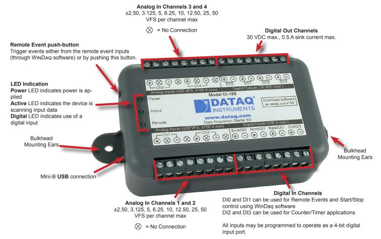
Screw terminals for signal inputs
