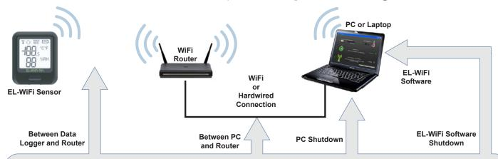
EL-WiFi products support a failsafe operation feature that ensures retained readings and data logging continuity in the event of failure at one or more communication junctions: between the data logger and the WiFi router; between the WiFi router and PC; PC shut down; EL-WiFi software shutdown.
